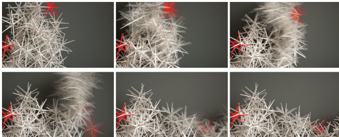
Figure 2. A designed granulate re-configures through an outside trigger from one stable state to the other.
